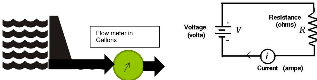
If we know the voltage and the resistance in a circuit, we can calculate the current that would be flowing using the following expression:
