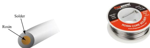
*Using acid core solder will cause the connection to eventually corrode and fail*
