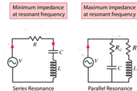
*Resonance occurs when the Capacitive reactance is equal to the inductive reactance*
