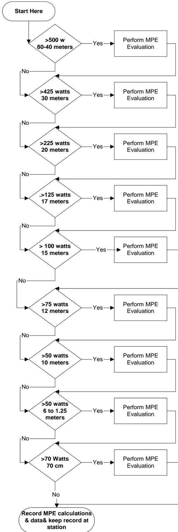
**Note- Decision for running MPE at any specific frequency is determined by the ERP which is the transmitter output power plus antenna gain minus any feed line losses, filter or other losses**
