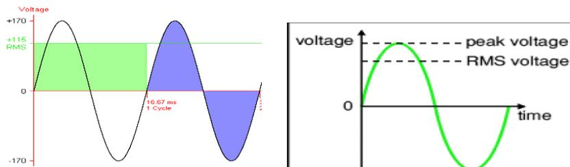
For a pure sine wave the equivalent RMS value is 0.707 times the peak value. Conversely the peak voltage can be calculated as 1.414 times the RMS Value.
