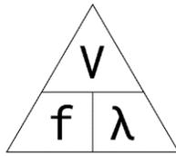
In amateur radio we frequently refer to our frequencies in terms of approximate wavelength. Since we frequently operating in the megahertz band we can simplify our conversion to wavelength by dividing the frequency in megahertz (MHz) into 300. For example:
