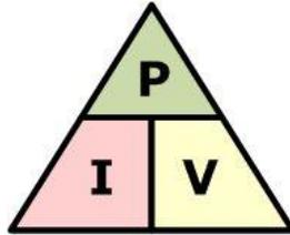
Power is work done by electricity and is defined as the voltage across a circuit multiplied by the current flowing through the circuit.
