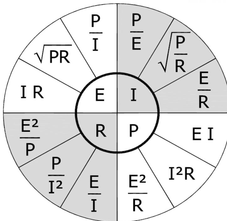
Units are E in Volts, R in Ohms, I in amperes, P in watts
